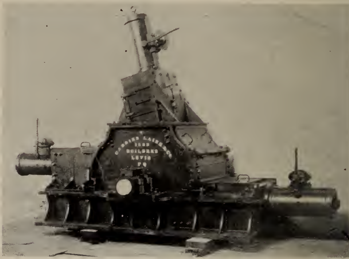
Fig. 20—Pulp grinder, manufactured by Carrier, Laine & Co.
